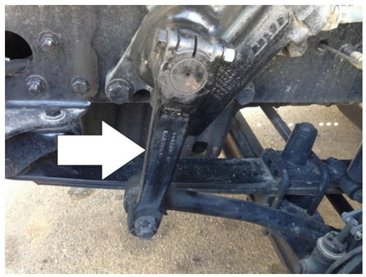
**<u>Drag Link</u>**Properly Mounted and Secure. Not Cracked, Bent, or Broken.
